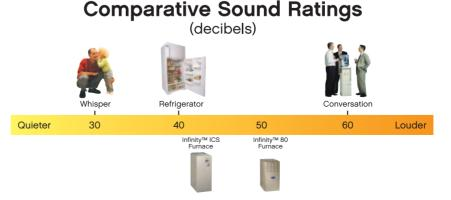
Carrier manufactures gas furnaces that are among the quietest in the industry. We test our products in a sound laboratory specifically built to mble a typical residence. Sound level recordings produced at steady state, low fire operation (the most common operating condition), measured 3 feet from furnace. Other sound levels, mentioned for comparison, as published at http://www.nidcd.nih.gov/health/hearing.ruler.asp.
