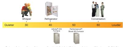
Carrier manufactures gas furnaces that are among the quietest in the industry. We test our products in a sound laboratory specifically built to resemble a typical residence. Sound level recordings produced at steady state, low fire operation (the most common operating condition), measured 3 feet from furnace. Other sound levels, mentioned for comparison, as published at http://www.nidcd.nih.gov/health/hearing.ruler.asp.
