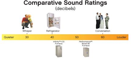
Carrier manufactures gas furnaces that are among the quietest in the industry. We test our products in a sound laboratory specifically built to resemble a typical residence. Sound level recordings produced at steady state, low fire operation (the most common operating condition), measured 3 feet from furnace. Other sound levels, mentioned for comparison, as published at http://www.nicdc.nih.gov/heurers.publicers.publicers.
