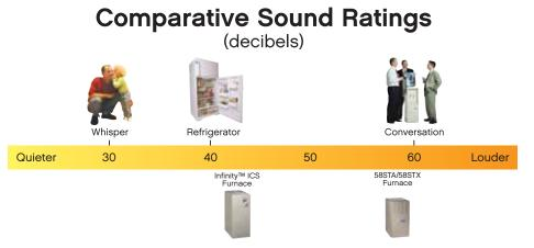
Carrier manufactures gas furnaces that are among the quietest in the industry. We test our products in a sound laboratory specifically built to esemble a typical residence. Sound level recordings produced at steady state, low fire operation (the most common operating condition), measured 3 feet from furnace. Other sound levels, mentioned for comparison, as published at http://www.nidcd.nih.gov/health/hearing.ruler.asp.
