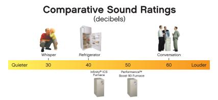
Carrier manufactures gas furnaces that are among the quietest in the industry. We test our products in a sound laboratory specifically built to resemble a typical residence. Sound level recordings produced at steady state, low fire operation (the most common operating condition), measured 3 feet from furnace. Other sound levels, mentioned for comparison, as published at http://www.nidcd.nih.gov/health/hearing.ruler.osp.
