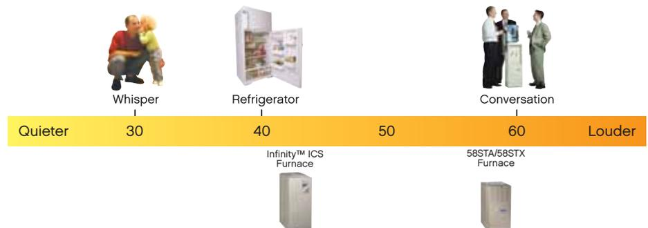
Carrier manufactures gas furnaces that are among the quietest in the industry. We test our products in a sound laboratory specifically built to resemble a typical residence. Sound level recordings produced at steady state, low fire operation (the most common operating condition), measured 3 feet from furnace. Other sound levels, mentioned for comparison, as published at <http://www.nidcd.nih.gov/health/hearing/ruler.asp>.
